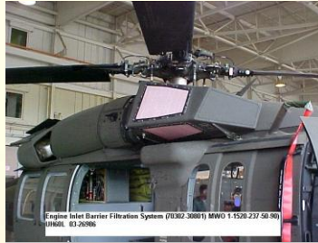
Engine Inlet Barrier Filter "OIF Threshold"
